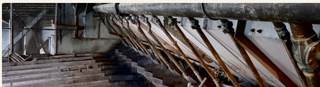
THE BUCKET LINE: SEVENTY-ONE BUCKETS, EIGHT CUBIC FEET APIECE
